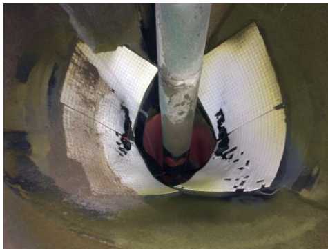
Above: Photo showing the worn ceramic lining trialled inside the wok. Below: photo of worn rubber lining
