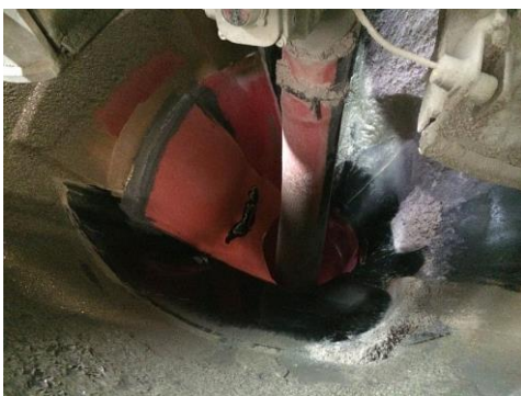
Above: Photo showing the worn ceramic lining trialled inside the wok. Below: photo of worn rubber lining
