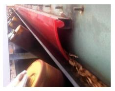
The customer has now installed the K-Snap-Loc® Dust Deal System. The superior low friction properties of the engineered polyurethane has immediately prevented any further signs of wear to the belt covers. By maximising the efficiency in the materials conveyed and providing effective spillage, the investment in Kinder Australia's K-Snap-Loc® Dust Seal System has long term benefits.
