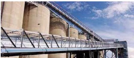
*Photos of K-Snap-Loc installed around the transfer point – the blue polyurethane indicates the Fire Resistant Anti Static FRAS properties.*
