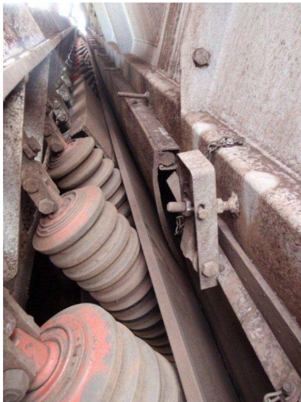
Photo taken February 2013 of K-Snap-Loc Dust Seal System in place on slider beds at the Power Station, Traralgon, Victoria
