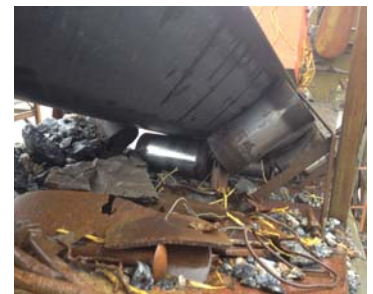
Images of conveyor damage resulting from incorrect frame maintenance
