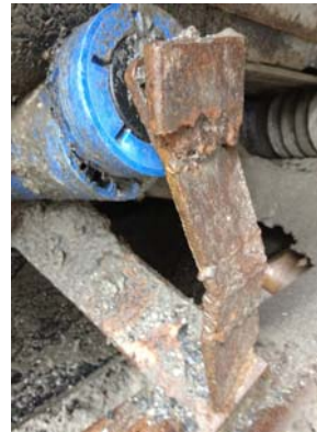
Images of conveyor damage resulting from incorrect frame maintenance
